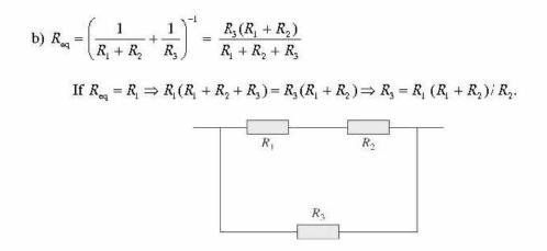
**26.49**: a) We wanted a total resistance of 400  $\Omega$  and power of 2.4 W from a combination of individual resistors of 400  $\Omega$  and 1.2 W power - rating.
